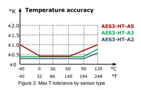
Note on accuracy: allow one hour after power up for compensation swing in
