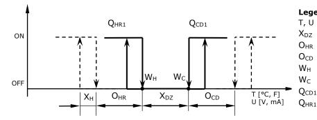
LegendT, UInput signalXDZDead zoneOHROffset heating/reverseOCDOffset cooling/directWHSet point heating/reverseWCSet point cooling/directQCD1Binary sequences cooling/directQHR1Binary sequences heating/reverse
